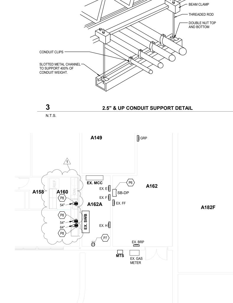
FIRST FLOOR POWER PLAN - ELECTRICAL ROOM SCALE: 1/8" = 1'-0"
