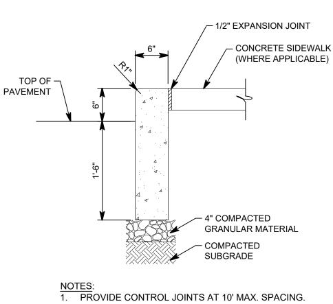
NOTES: 1. PROVIDE CONTROL JOINTS AT 10' MAX. SPACING. 2. PROVIDE EXPANSION JOINTS AT 80' MAX. SPACING AND AT ENDS OF ALL RADII.
