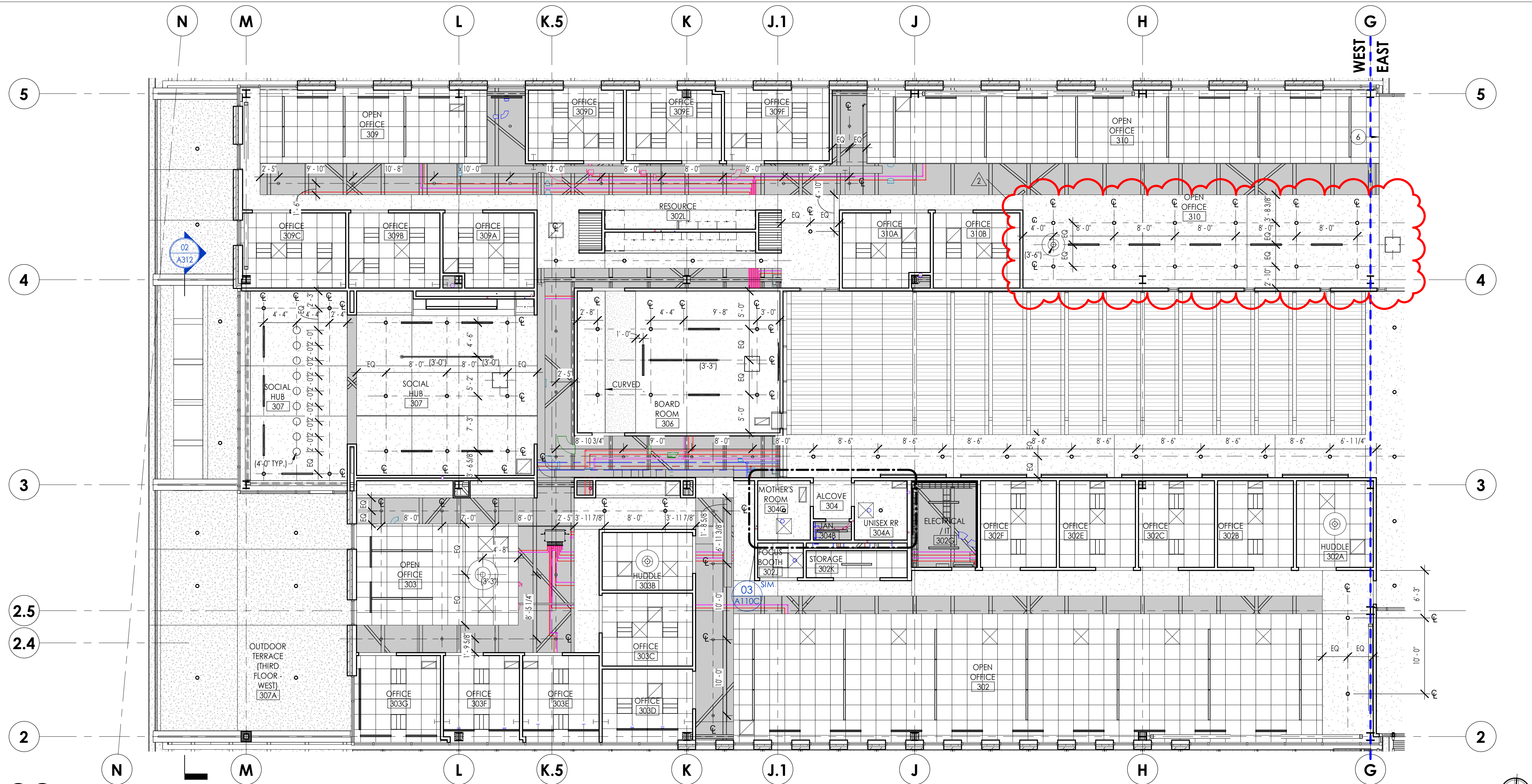
02 THIRD FLOOR REFLECTED CEILING PLAN - WEST - LIGHTING SCALE: 1/8" = 1'-0"
