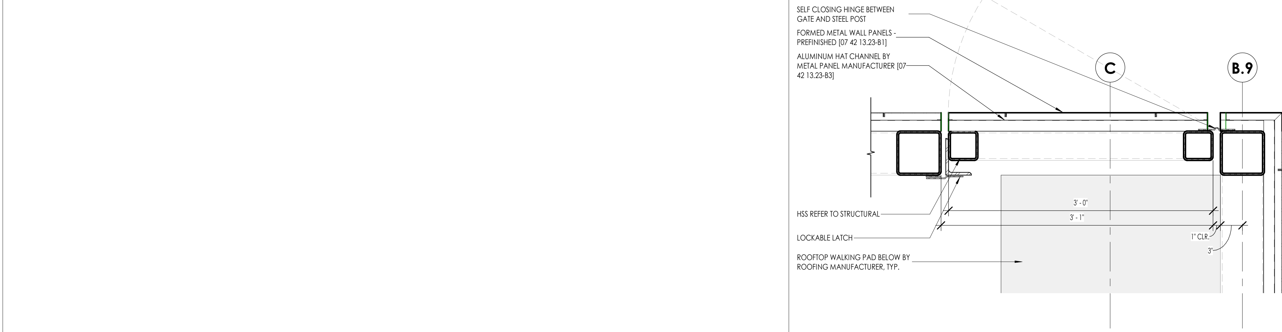
07 ROOF SCREEN DOOR SCALE: 1 1/2" = 1'-0"
