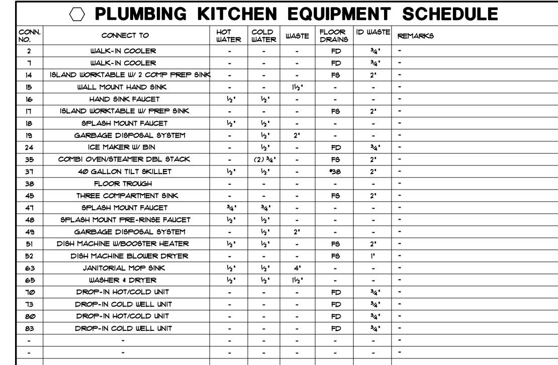
THIS CONTRACTOR SHALL PROVIDE ALL ROUGH-IN AND FINAL SERVICES AND CONNECT ALL WATER LINES, WASTE LINES, INDIRECT PIPING, ETC. FOR FIXTURES AND KITCHEN EQUIPMENT ITEMS. PROVIDE AND INSTALL ALL YALVES, STOPS, TRAPS, AND PRESSURE REGULATORS NECESSARY TO CONNECT LINES. FOR FURTHER INFORMATION AND DESCRIPTION OF KITCHEN EQUIPMENT BEING SUPPLIED REFER TO ARCHITECTURAL DRAWINGS, KITCHEN EQUIPMENT DRAWINGS, AND ENLARGED KITCHEN AREA DRAWINGS.
