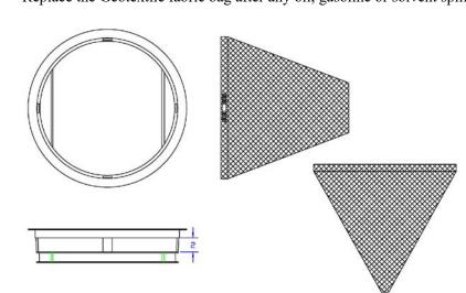
UENERAL NUTES: FRAME: Top flange fabricated from 1½"x1½"x½" angle. Base rim fabricated from 1½"x½"x½" channel. Handles and suspension brackets fabricated from 1¼"x½" flat stock. All steel conforming to ASTM-A36. SEDIMENT BAG: Bag fabricated from 4 oz./sq.yd. non-woven polypropylene geotextile reinforced with polyester mesh. Bag secured to base rim with a stainless steel band and lock.
