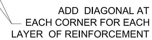
6 CONCRETE REINFORCEMENT AT OPENINGS DETAIL
