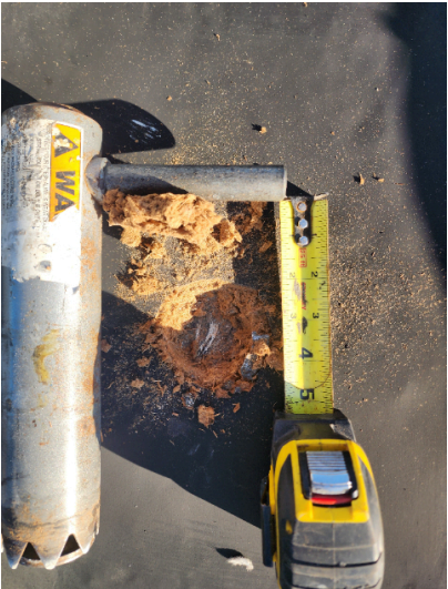
Section 2 Lightweight concrete (Flat) .5" Wood fiber EPDM adhered
